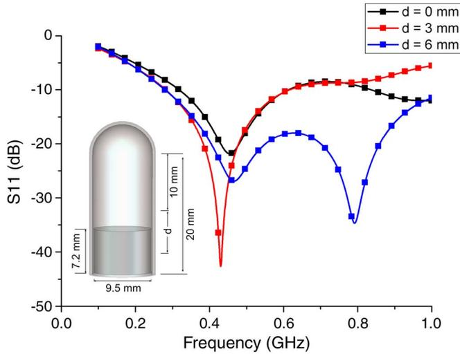
Fig. 4. Simulated return loss with battery in various positions. (*d*: distance from the center of cylindrical capsule face to the center of the battery).
