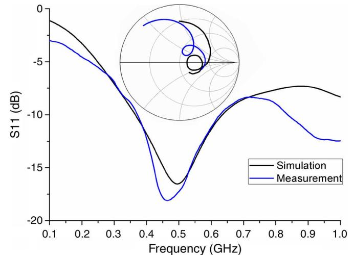
Fig. 3. Comparison between simulated return loss and measured return loss.
