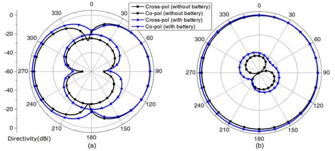
Fig. 6. Simulated radiation patterns of proposed antenna in (a) *xy*-cut plane and (b) *yz*-cut plane.
