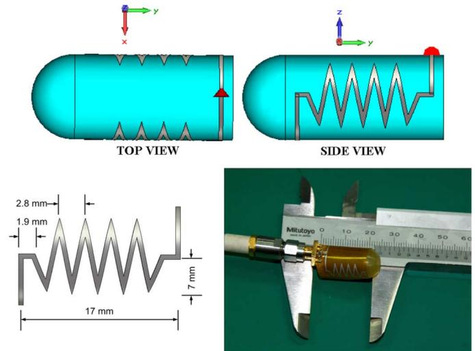
Fig. 2. Proposed outer-wall loop antenna.
