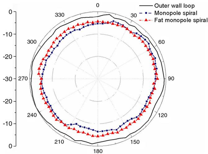
Fig. 9. Normalized measured power of receiving antenna.
