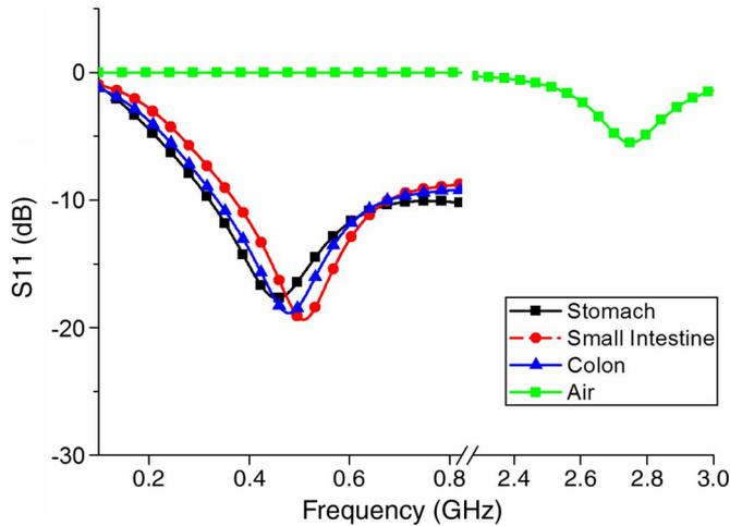
Fig. 5. Simulated return loss in various tissues.
